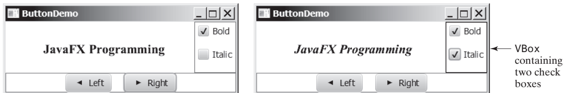
FIGURE 16.8 The program demonstrates check boxes. Source: Copyright © 1995–2016 Oracle and/or its affiliates. All rights reserved. Used with permission.
