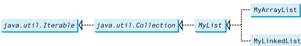
FIGURE 24.2 MyList defines a common interface for MyArrayList and MyLinkedList .
