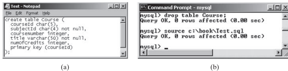
FIGURE 34.11 (a) You can use Notepad to create a text file for SQL commands. (b) You can run the SQL commands in a script file from MySQL.
