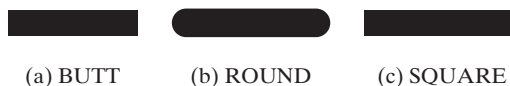
FIGURE 31.15 (a) No decoration for a BUTT line cap. (b) A half circle is added to an unclosed path. (c) A square with half of the stroke width is extended to an unclosed path.
