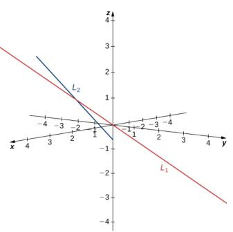
c. Lines  $L_1$  and  $L_2$  have equivalent direction vectors:  $\mathbf{v} = \langle 6, -2, 3 \rangle$ . These two lines are parallel (see the following figure).
