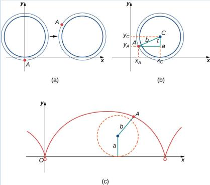
**Figure 1.15** (a) The ant is hanging onto the flange of the train wheel. (b) The new setup, now that the ant has jumped onto the train wheel. (c) The ant travels along a prolate cycloid.
