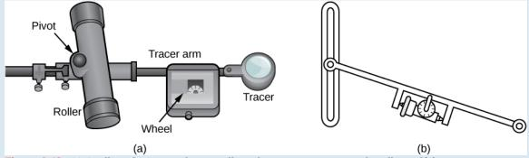
**Figure 6.48** (a) A rolling planimeter. The pivot allows the tracer arm to rotate. The roller itself does not rotate; it only moves back and forth. (b) An interior view of a rolling planimeter. Notice that the wheel cannot turn if the planimeter is moving back and forth with the tracer arm perpendicular to the roller.
