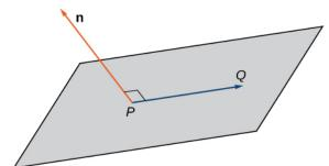
**Figure 2.69** Given a point P and vector  $\mathbf{n}$ , the set of all points Q with  $\overrightarrow{PQ}$  orthogonal to  $\mathbf{n}$  forms a plane.
