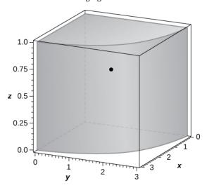
**339**. a.  $\bar{x} = \frac{3\sqrt{2}}{2\pi}$ ,  $\bar{y} = \frac{3(2-\sqrt{2})}{2\pi}$ ,  $\bar{z} = 0$ ; b. the solid Q and its center of mass are shown in the following figure.
