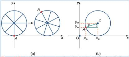
**Figure 1.13** (a) The ant clings to the edge of the bicycle tire as the tire rolls along the ground. (b) Using geometry to determine the position of the ant after the tire has rotated through an angle of t.
