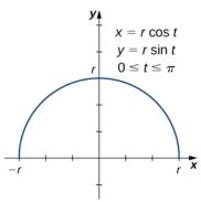
**Figure 1.26** A semicircle generated by parametric equations.
