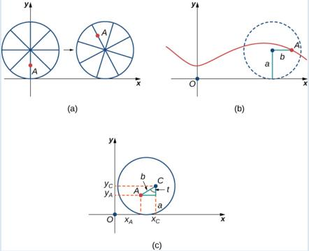
**Figure 1.14** (a) The ant climbs up one of the spokes toward the center of the wheel. (b) The ant's path of motion after he climbs closer to the center of the wheel. This is called a curtate cycloid. (c) The new setup, now that the ant has moved closer to the center of the wheel.
