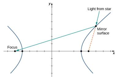
Figure 7.53 A hyperbolic mirror used to collect light from distant stars.
