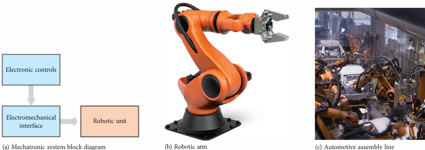
FIGURE 1-5 Example of a mechatronic system and application. Part (b) Beawolf/Fotolia; Part (c) Small Town Studio/Fotolia.
