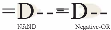
FIGURE 3-30 ANSI/IEEE standard symbols representing the two equivalent operations of a NAND gate.
