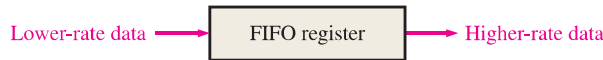
(b) Data input at a slow keyboard rate can be stored and then transferred at a higher rate for processing.
