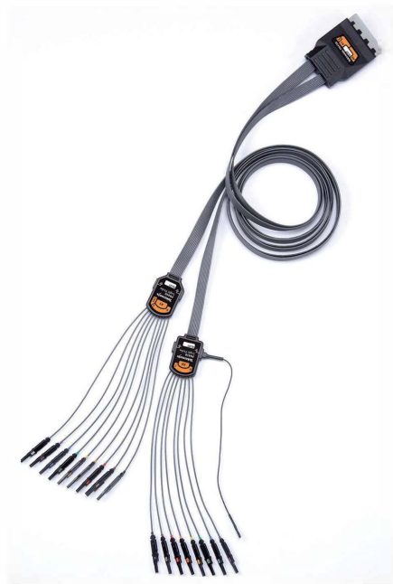
FIGURE 1-53 A typical multichannel logic analyzer probe. Used with permission from Tektronix, Inc.
