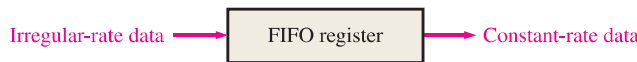
(a) Irregular telemetry data can be stored and retransmitted at a constant rate.
